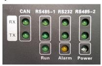
The LED indicators in the above picture are mainly devided into two parts: indicator of status (operation, alarm, power) and indicator of communication (CAN, RS485, RS2332). Working status for the indicators are shown in the following list.
